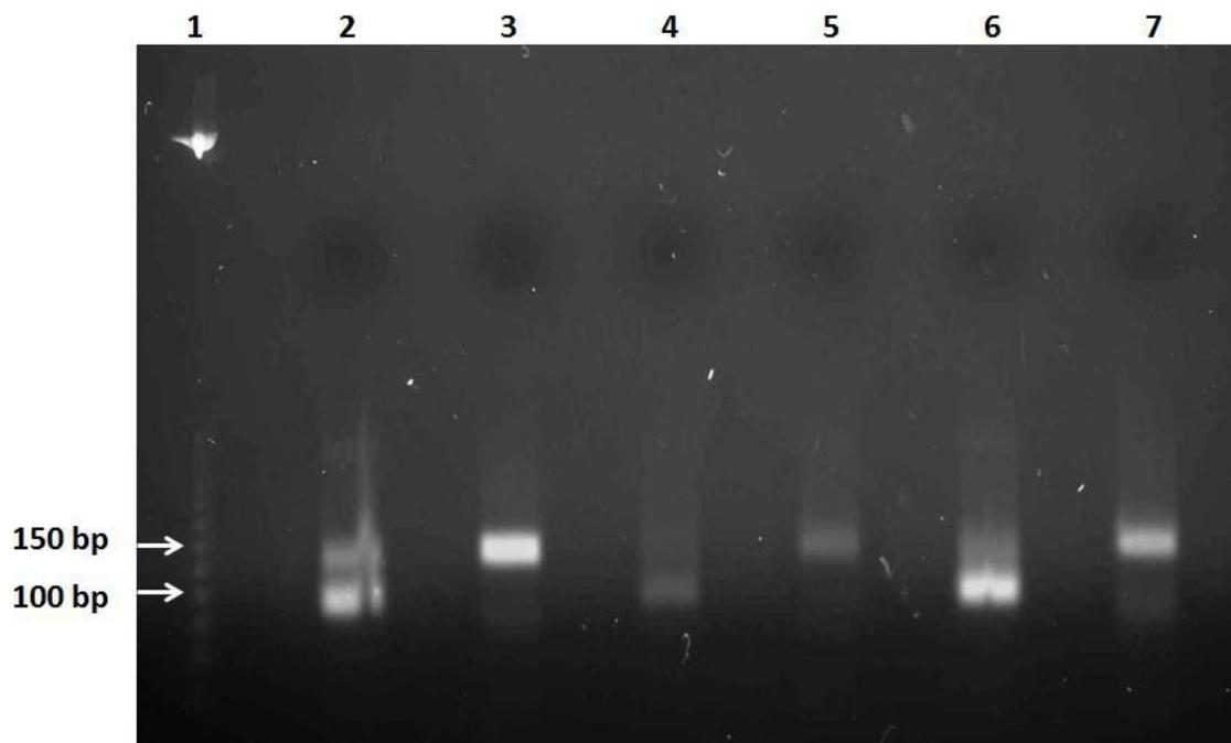
**Figure 5:** PCR amplification of the DpnII digest. 1) 25 bp DNA step ladder; 2) non-digested DNA P1 + P2 primers; 3) non-digested DNA P1 + P3 primers; 4) digested DNA heat-inactivated sample P1 + P2 primers; 5) digested DNA heat-inactivated sample P1 + P3 primers; 6) digested DNA precipitated sample P1 + P2 primers; 7) digested DNA precipitated sample P1 + P3 primers.
